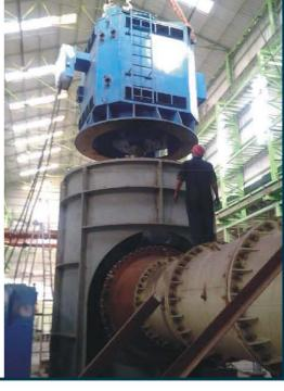
Pump Model Study for Upper Bhadra Lift Irrigation Scheme of Karnataka Neeravari Nigam Ltd. - Pump: 2000 MVC, Discharge: 43,200 m3/hr, Head: 44.5 mtrs., Speed: 370 rpm
